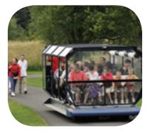
28 seats including 1 for PRM 3 electric vehicles Radar anti-collision system GPS guidance system Silent
